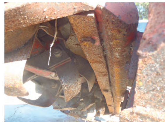
Figure 5. Side operating tree hoe: side view (top photo) and cultivator tines seen from below (bottom photo). Photo credit: Phil Stansly
